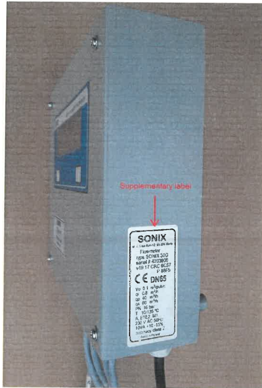
Fig 7, supplementary label on right side of transducer case
